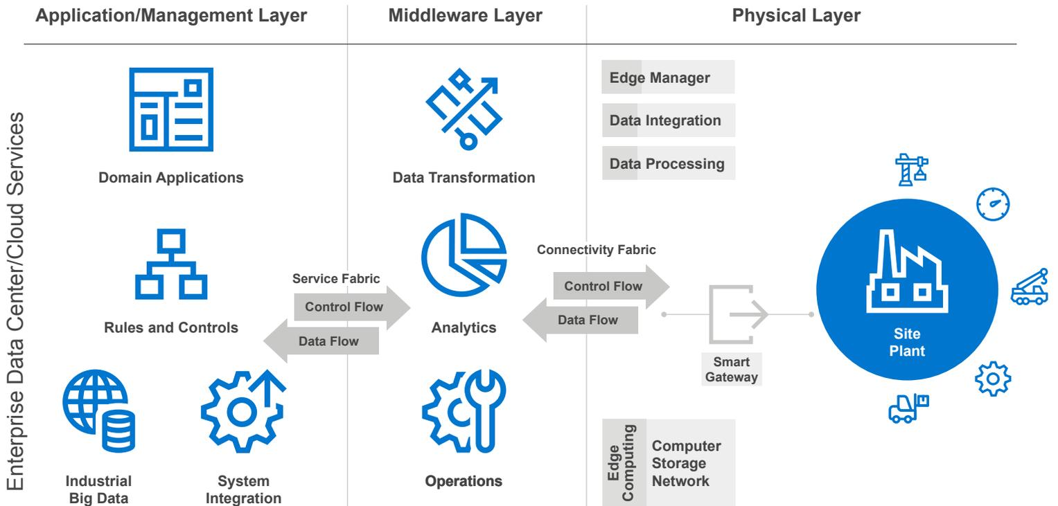
Fig 3. IloT Edge Computing Reference Architecture
